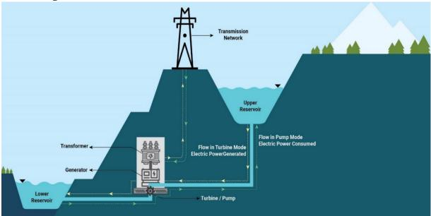
Figure 1: A pumped-hydro energy storage (PHES) system
