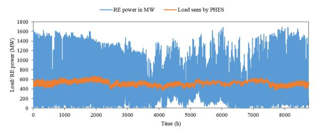
Figure 13: RE profile (both solar and wind) at the Pinnapuram RE plant and normalised load as seen by the PHES for a year
