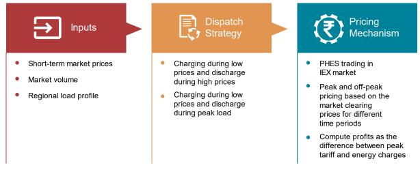
Figure 7: Tariff computation method for energy arbitrage/peak-load shaving/load following
